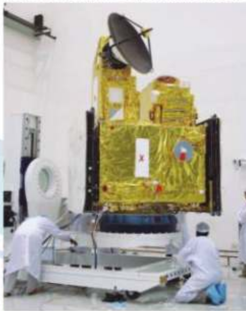
Oceansat-2 being prepared for prelaunch tests
