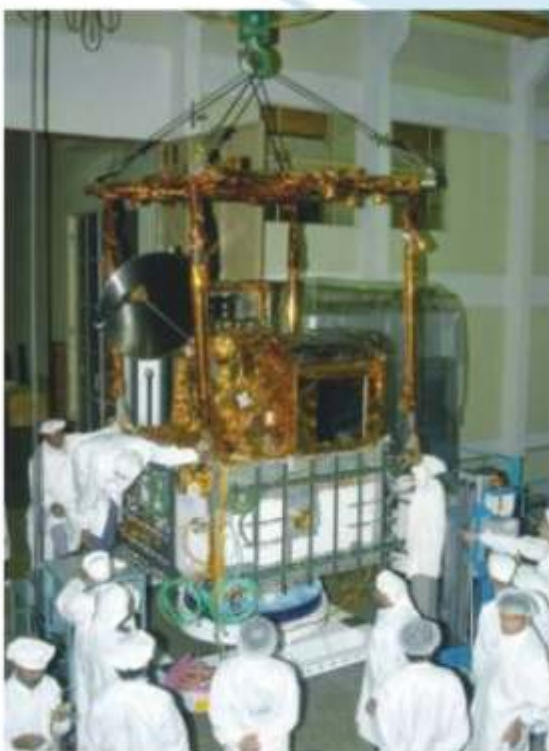
Readying Oceansat-2 for Thermo-vacuum test
