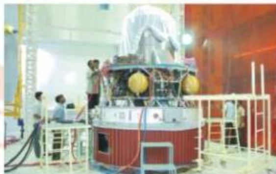
Launch vehicle personnel working on PSLV-C14 fourth stage
